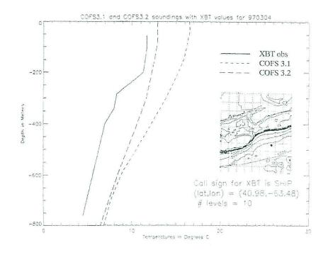
March 4, 1997 are compared. Again, much better agreement with the observed profile is seen for the case where data assimilation has been included even though the lack of agreement at deeper levels still persists. Some of the disagreement may be attributed to factors such as parameterization of mixing and lateral boundary conditions.
