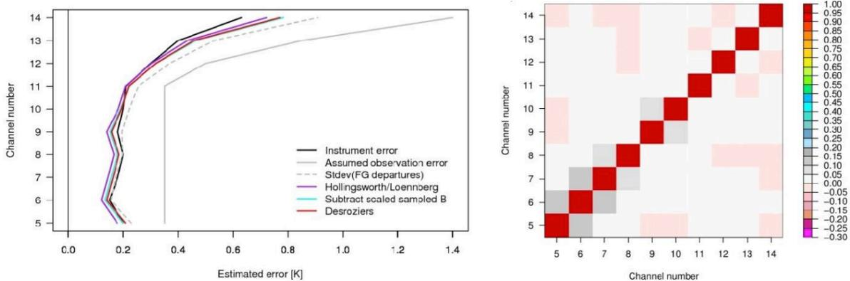
Figure 2: (left) Estimates of  $\sigma_o$  for AMSU-A on NOAA-18 from the Hollingsworth/Lönnberg (purple) and Desroziers (red) diagnostics, together with estimates of the instrument noise (black), the standard deviation of background departures (dashed grey), and the observation error assumed in 2008 (grey). (right) Estimates of observation error correlations obtained with the Desroziers diagnostic.
